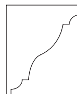
SG.H.2117: Under-eave cornice Height 214 mm Depth 168 mm Length 1000 mm
